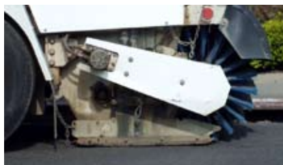
The curvature in the broom furrows material toward the center of the elevator and helps minimize trailing.
